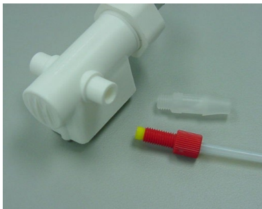
Example of \frac{1}{4} -28 UNF bottom sealing fitting (bottom) and face sealing fitting (top)
