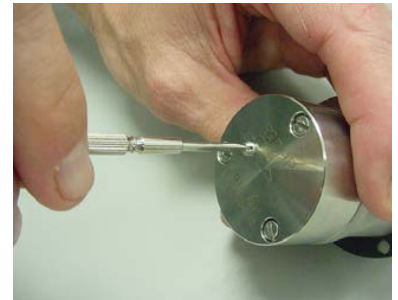
Internal pressure-relief valve: turn clockwise to close, counter-clockwise to open.
